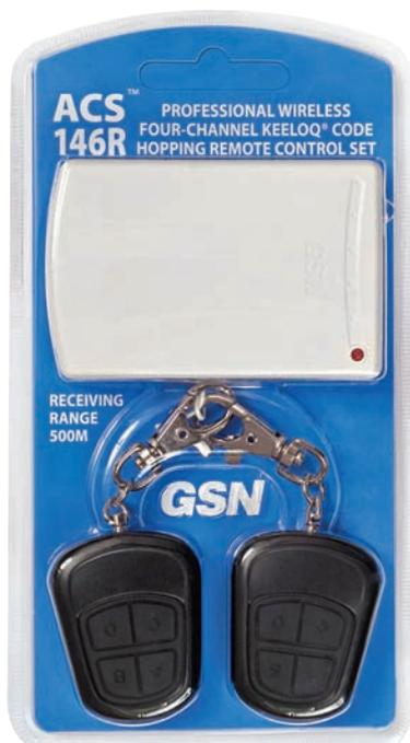
**ACS 146R - wireless four-channel multifunctional receiver, operating in conjunction with two hand-held push button transmitters, providing the remote control of any electronic equipment:**
